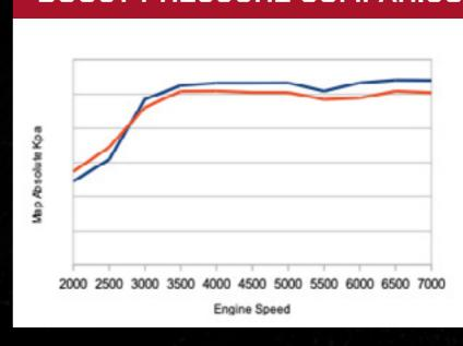
He increase in the duty cycle of the high-pressure petrol pump can be quantified at around 3%, with a maximum peak of 4%, thanks to the greater demand for fuel due to the higher boost pressure. This increase in boost pressure can therefore be generated by the improved ability to draw air in thanks to the permeable air filter and an adjustment of the intake air flow given by the design of the Sprint Filter C-Tech airbox.
